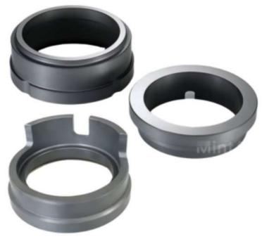
Sintered Silicon Carbide offers a high-performance seal face material that has proven successful in such diverse pumping applications as chemical processing, refining, mining and pulp and paper processing. The material provides superior corrosion and abrasion resistance; shock resistance; and low sliding friction against a wide range of mating materials
